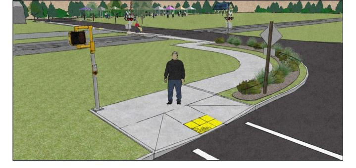
A key gap in the existing Sawmills sidewalk network is between Sawmills School Road and Highway 321A. This view shows a sidewalk extending around the corner of 321A toward the Caldwell County Railroad. The rendering shows a new sidewalk, with an ADA-compliant railroad crossing and pedestrian ramp, extending along Sawmills School Road toward the Farmers Market Rendering by Duncan Cavanaugh.
