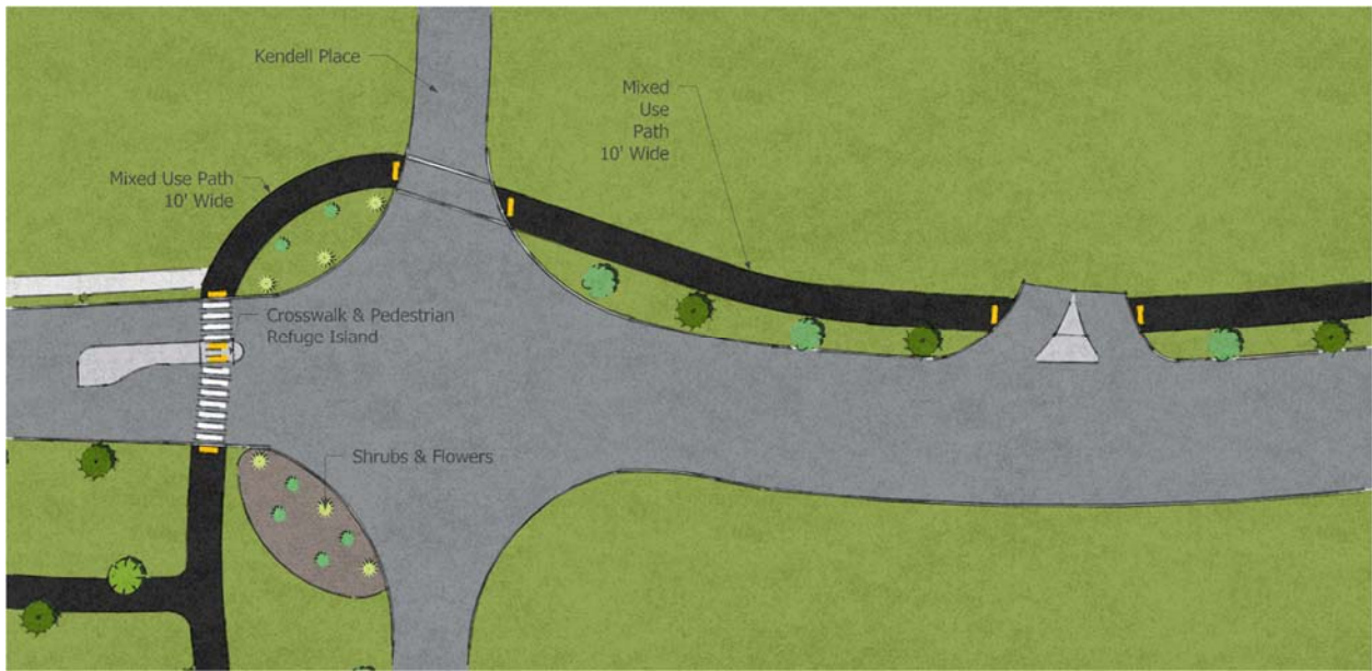
This close-up drawing shows a pedestrian crosswalk and a pedestrian refuge island at the Cahaj Mountain Road/Kendell Place/Helena Street intersection. A mixed-use path connects to a sidewalk on the north side of Cahaj Mountain Road, and continues to the east, via a pedestrian crosswalk extending across Kendell Place. Shrubs have been planted to encourage motorists to slow down and for visual appeal.
